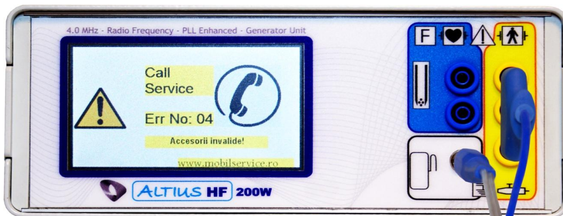
Figure no.32 – Alert on possible malfunctions
